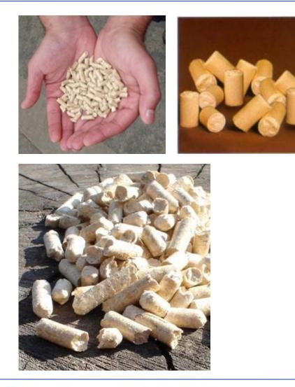
Granulated spin and sawdust D=5-10mm, L=10-25mm
